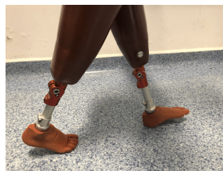
Figure 7: Child’s gait test with the new prosthetic feet.
